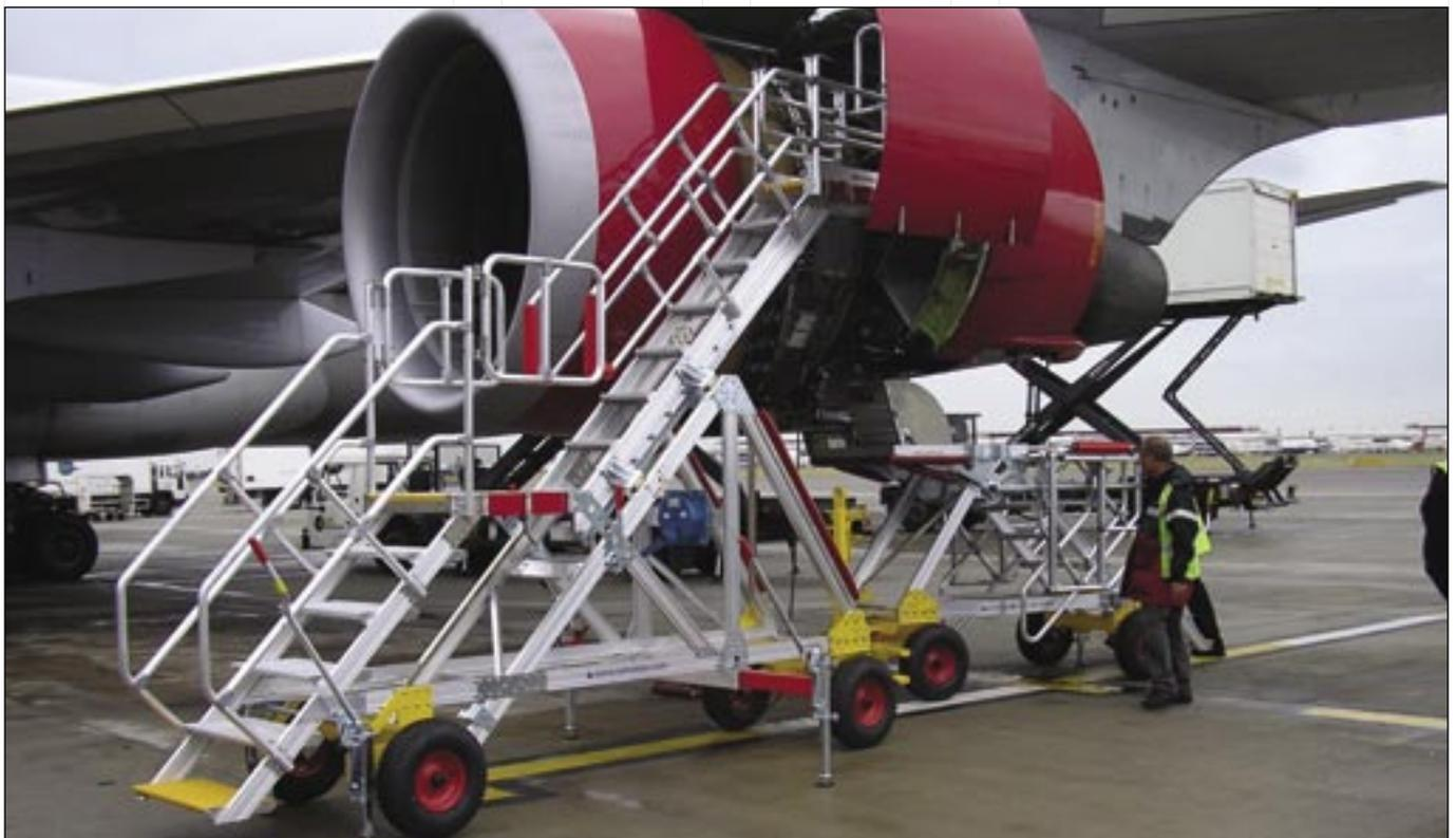
went back to the drawing board, and the supplier came up with another design using the same template as the existing steps, but we had to 'stretch' them slightly so they complied with the new standard. And in order to meet the new health and safety specifications, Semmco added some adjustable hand rails too.
